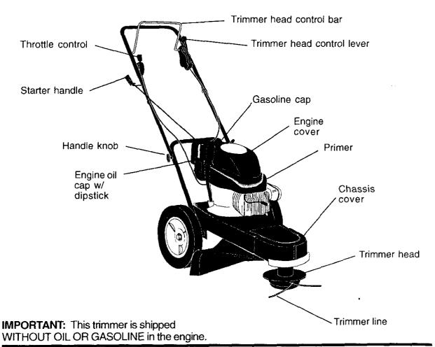
Trimmer head control bar - must be held down to the handle to engage trimmer head. Release to stop the trimmer head.
